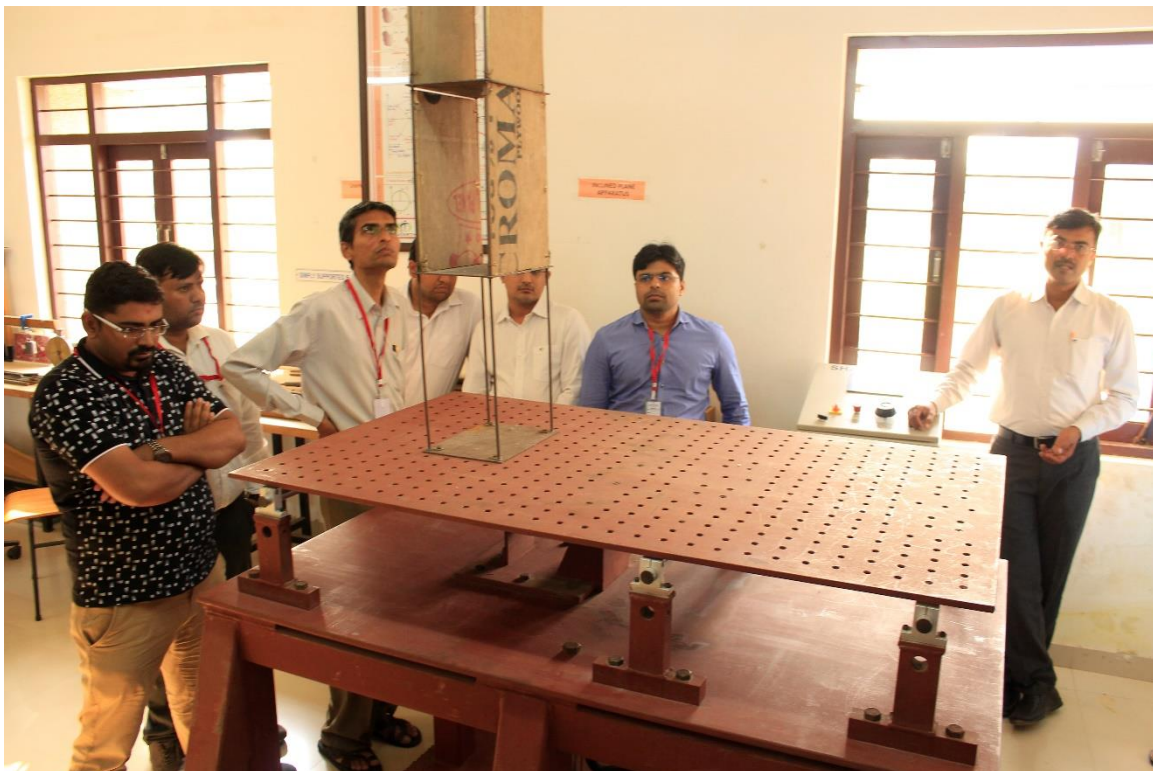
Glimpse 12 Demonstration of Seismic Table at the Institute as PLC based system by Dr. D. D. Vyas
